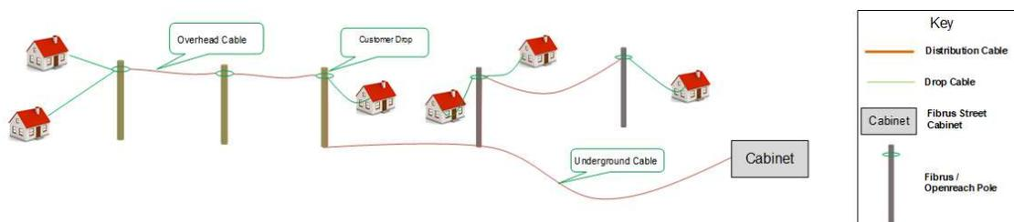
The majority of installation will be overhead, however in some cases we also use a combination of Fibrus and Openreach underground duct or simply the Openreach underground duct.
