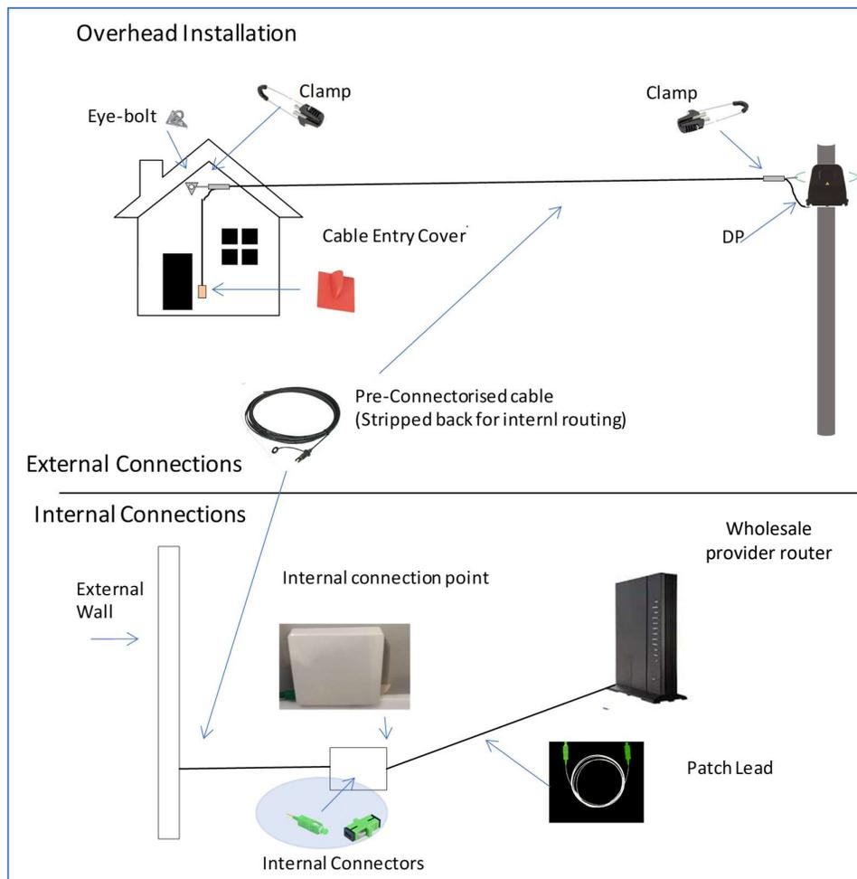
Our NTE must be fixed to a wall inside the property, close to a power socket. The external cable runs through a hole we will drill in the wall, down into the ground where it will then run back to connect to our network.
